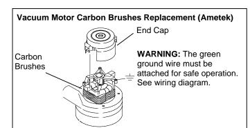
**Note:** When replacing carbon brushes loosen wire terminal **BEFORE** removing screws on bracket.
